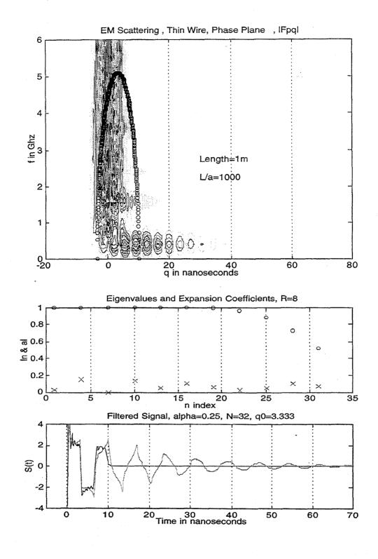
Figure II. Scattering from thin Wire. L=1m. L/a=1000. Angle of Incidence is 90°. R=8.
