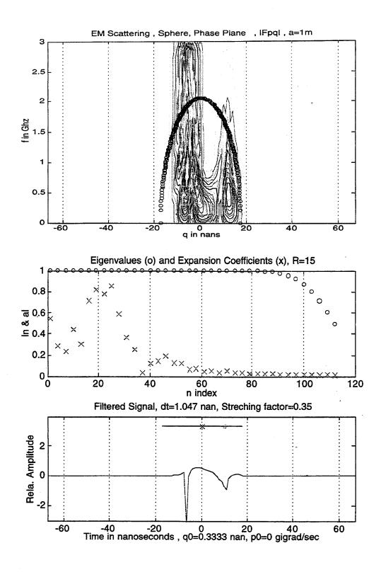
Figure L. Scaterring from a perfectly conducting Sphere. Radius =1 m. Filter Radius =10.
